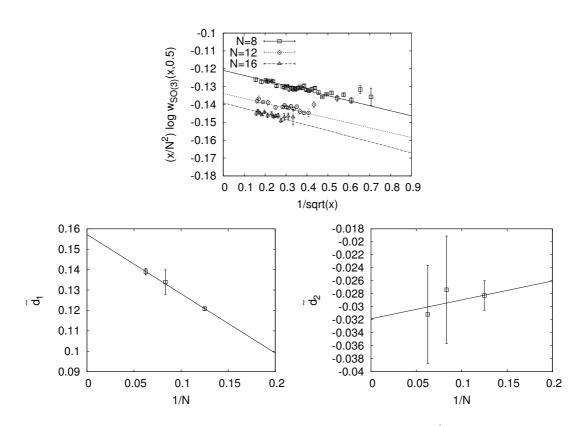
Figure 16. (Top) The function  $\frac{x}{N^2} \log w_{SO(3)}(x, 0.5)$  is plotted against  $\frac{1}{\sqrt{x}}$  for N = 8, 12, 16. The straight lines represent the fits to the asymptotic behavior (D.1). (Bottom) The coefficients  $\tilde{d}_1$  and  $\tilde{d}_2$  in the asymptotic behavior (D.1) extracted from the top figure are plotted against  $\frac{1}{N}$ . The data points can be fitted nicely to a straight line.
